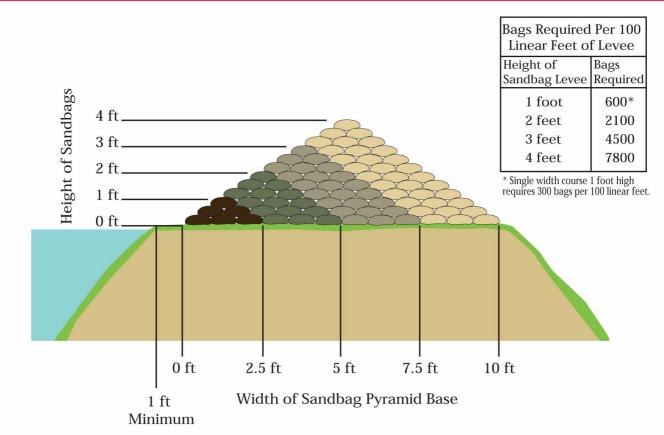
The pyramid placement method issued to increase the height of sandbag protection.
